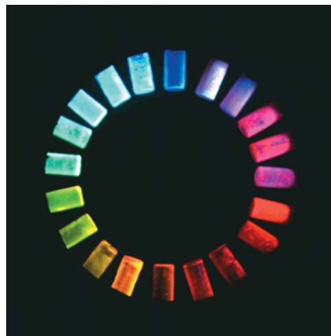
Figure 2. Cast films (from chloroform) of oligomers 1–15 under UV excitation ( \lambda_{\text{exc}} = 363 nm).
